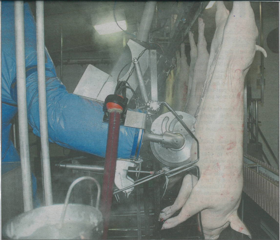
Australia's first laser-guided pork cutting robot at work at Craig Mostyn Group's Linley Valley Fresh processing works in Woorloo.
